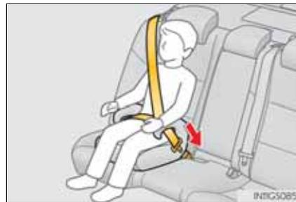
Check that the shoulder belt is correctly positioned over the child's shoulder and that the lap belt is as low as possible. (→P. 38)
