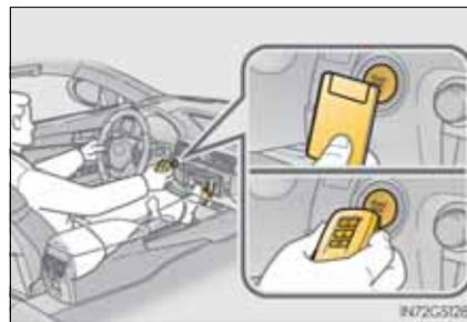
3 Firmly depress the brake pedal and check that
