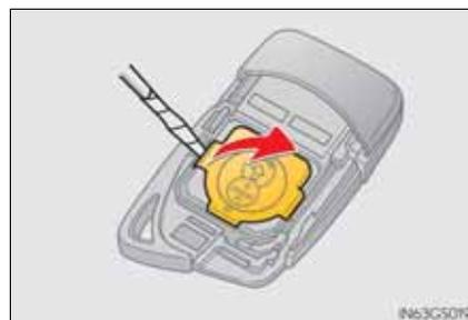
**4 Remove the depleted battery.**
