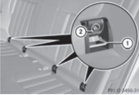
When installing the LATCH-type (ISOFIX) child restraint system, fold protective caps ② of LATCH-type (ISOFIX) securing rings ① inwards.
