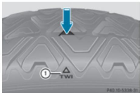
Bar indicator ① for tread wear is integrated into the tire tread.
