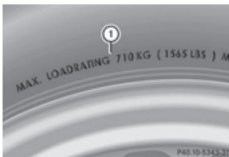
Maximum tire load **1** is the maximum permissible weight for which the tire is approved. Do not overload the tires by exceeding the specified load limit. The maximum permissi-
