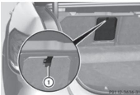
The through-loading facility is opened from the trunk.
