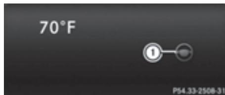
If Steering Assist and Stop&Go Pilot are activated but not ready for a steering intervention, steering wheel symbol ① appears in gray. If the system provides you with support by means of steering interventions, symbol ① is shown in green.
