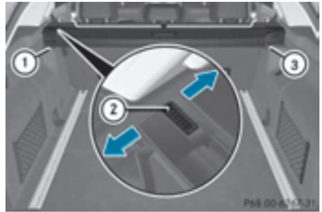
You can reach the combined cargo cover and net to install and remove it from the cargo compartment and, with the seat backrest folded forwards, from the left-hand rear door.
