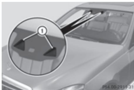
DISTRONIC PLUS with Steering Assist and Stop&Go Pilot aids you in keeping the vehicle in the center of the driving lane by means of moderate steering interventions in the speed range from 0 - 125 mph (0 - 200 km/h).
