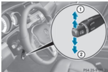
► Press the cruise control lever up ① for a higher speed or down ② for a lower speed.
