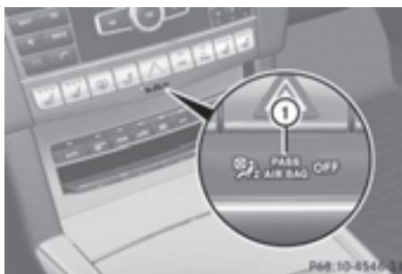
The PASSENGER AIR BAG OFF indicator lamp shows you whether the front-passenger front air bag is disabled.
