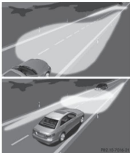
You can use this function to set the headlamps to change between low beam and high beam automatically. The system recognizes vehicles with their lights on, either approaching from the opposite direction or traveling in front of your vehicle, and consequently switches the headlamps from high beam to low beam.
