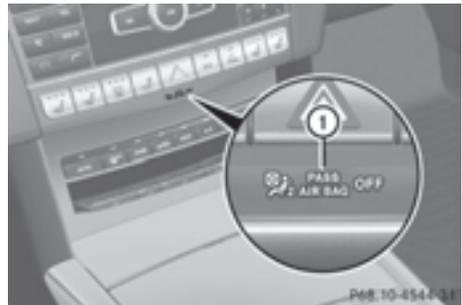
PASSENGER AIR BAG OFF indicator lamp ① is part of the Occupant Classification System (OCS).
