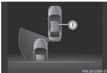
If a course-correcting brake application occurs, red warning lamp ① flashes in the exterior mirror and a dual warning tone sounds. In addition, display ② appears in the multifunction display underlining the danger of a side collision.
