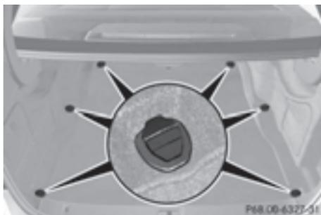
On vehicles without a through-loading feature in the rear bench seat, six plastic hooks are installed to the trunk floor.
