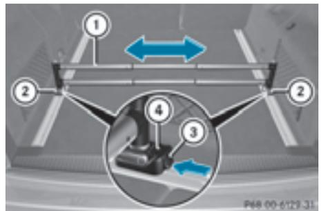
The telescopic rod can be used to secure the load against the rear seats to prevent it from moving around.
