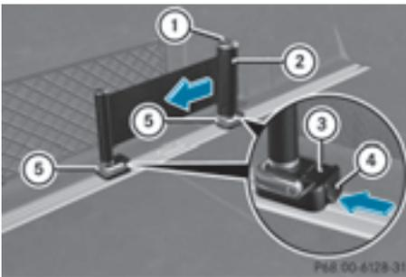
The luggage holder can be used to secure light loads against the side wall of the cargo compartment to prevent them from moving around.
