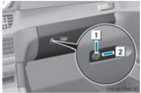
The glove box can only be locked and unlocked using the mechanical key.
