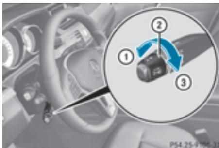
You can set the specified minimum distance for DISTRONIC PLUS by varying the time span between one and two seconds. With this function, you can set the minimum distance that DISTRONIC PLUS keeps to the vehicle in front, dependent on vehicle speed. You can see this distance in the multifunction display (▷ page 195).
