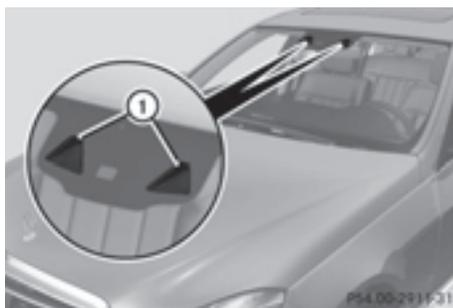
Lane Keeping Assist monitors the area in front of your vehicle with camera ①, which is mounted at the top of the windshield. Active Lane Keeping Assist detects lane markings on the road and can warn you before you leave your lane unintentionally.
