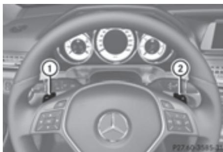
In the manual drive program, you can change gears manually using steering wheel paddle shifters ① and ②.
