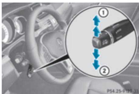
You can accept the current speed if you are driving faster than 20 mph (30 km/h).
