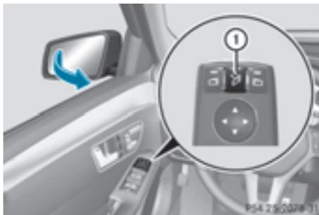
If you have switched on the **Auto. Mirror Folding** function and you fold in the exterior mirrors by pressing button ①, the exterior mirrors will not fold out automatically (▷ page 123).
