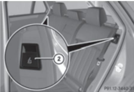
The left-hand and right-hand rear seat backrests can be folded forwards separately to increase the cargo compartment capacity. The combined cargo cover and net can remain installed.
