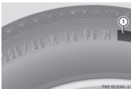
In addition to the load bearing index, load index **1** may be imprinted after the letters that identify speed index **6** on the sidewall of the tire (▷ page 378).
