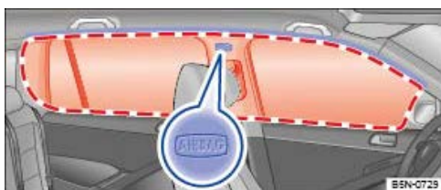
Fig. 20 On the left-hand side of the vehicle: location and deployment zone of the curtain airbag.
