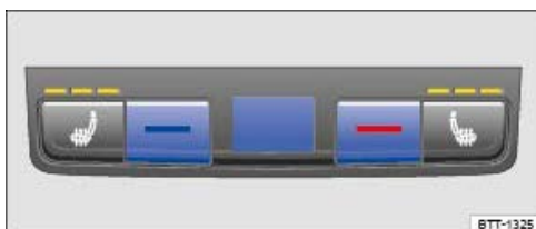
Fig. 123 In the rear centre console: controls for setting the temperature for the rear seats.
