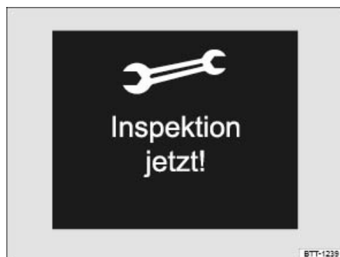
Fig. 56 In the instrument cluster display: example of a display in the instrument cluster when a service is due (illustration).
