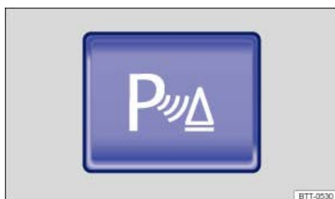
Fig. 175 In the centre console: button for switching the ParkPilot on and off (in some models).
