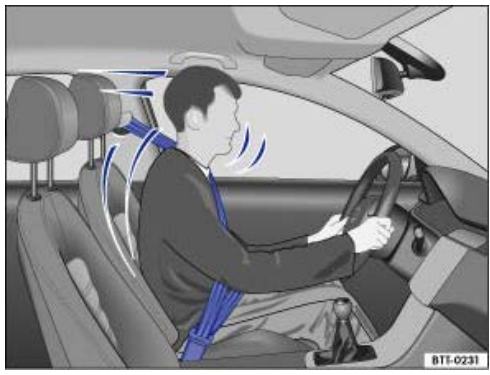
Fig. 8 Driver restrained by a properly positioned seat belt during a sudden braking manoeuvre.
