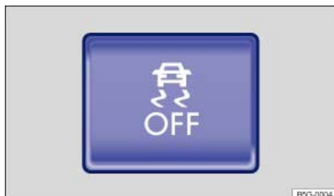
Fig. 195 In the lower part of the centre console: button for switching traction control system, traction control system with Electronic Stability Control or ESC Sport on and off manually.
