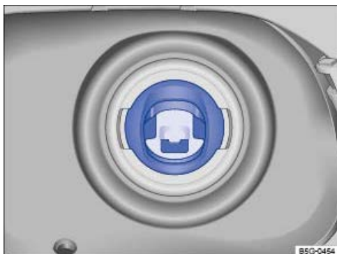
Fig. 229 Illustration: misfuelling prevention device in the tank filler neck.
