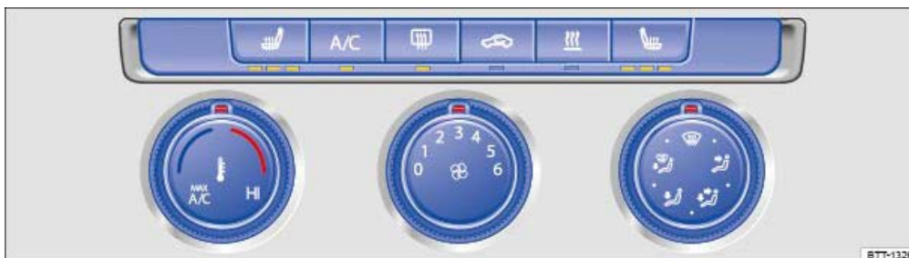
Fig. 121 In the upper part of the centre console: controls for the manual air conditioning system and/or heating and fresh air system.
