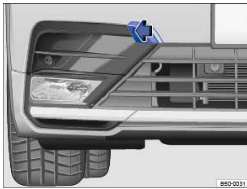
Fig. 250 In the right-hand side of the front bumper: cover for the towing eye mounting.
