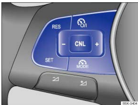
Fig. 153 Left-hand side of the multifunction steering wheel: buttons for operating the cruise control system.
