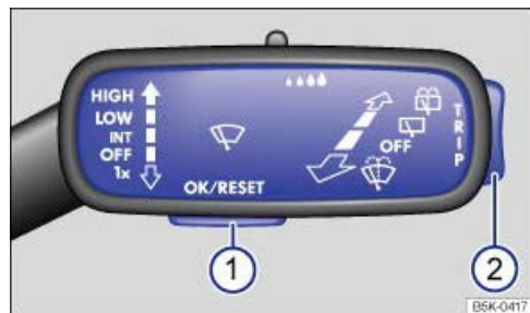
Fig. 58 On the right of the steering column: buttons on the wiper lever (vehicles without multifunction steering wheel).
