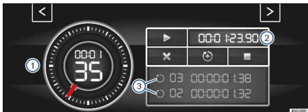
Fig. 62 On the infotainment system display: lap timer with stopwatch, function button and lap times.
