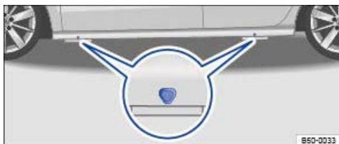
Fig. 276 Lifting points for the jack.
