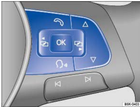
Fig. 59 Right-hand side of the multifunction steering wheel: buttons for using the menus and information displays in the instrument cluster display.
