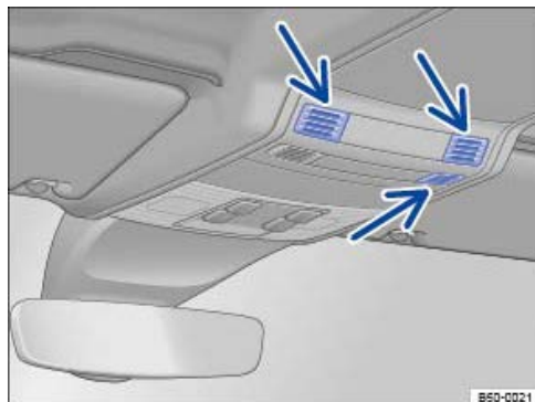
Fig. 73 In the roof console: sensors for the interior monitoring system (arrows).
