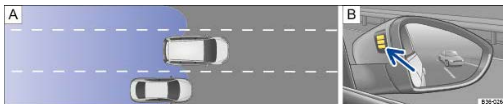
Fig. 171 Driving situation when overtaking and changing lanes. Visual display in the right-hand exterior mirror.
