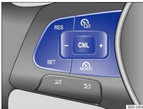
Fig. 156 Left-hand side of the multifunction steering wheel: buttons for operating the speed limiter.
