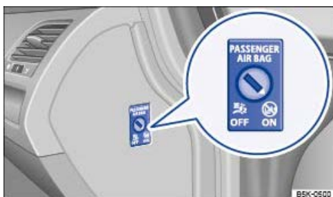
Fig. 17 In the dash panel on the front passenger side: key-operated switch for switching the front passenger front airbag on and off.
