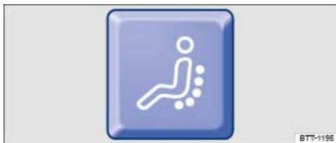
Fig. 107 In the lower area of the driver seat: button for massage function.
