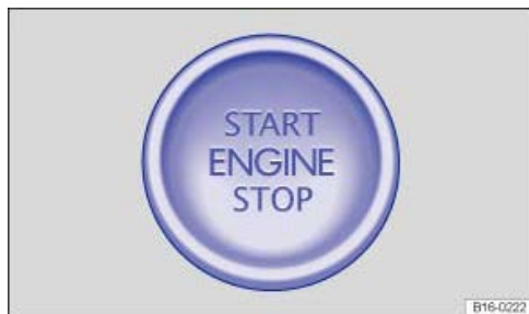
Fig. 134 In the lower section of the centre console: starter button for switching on the engine.
