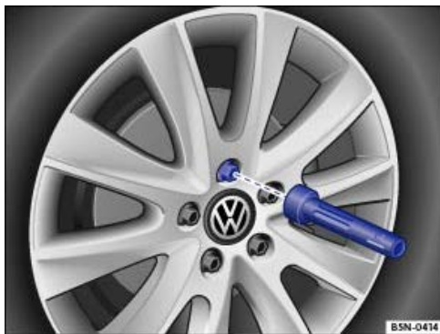
Fig. 278 Changing the wheel: removing the wheel bolts with the screwdriver handle.
