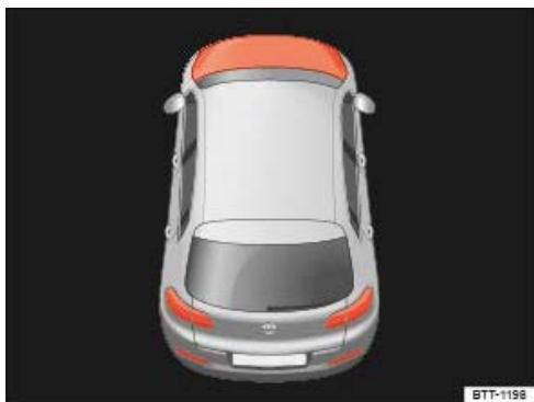
Fig. 255 On the instrument cluster display: the bonnet is open or not closed properly (illustration).
