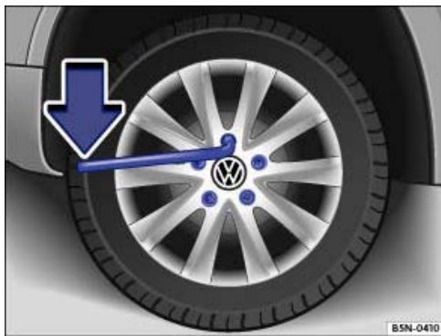
Fig. 274 Changing a wheel: loosening the wheel bolts.
