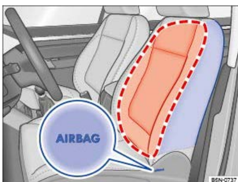
Fig. 19 On the side of the front seat: location and deployment zone of the side airbag.
