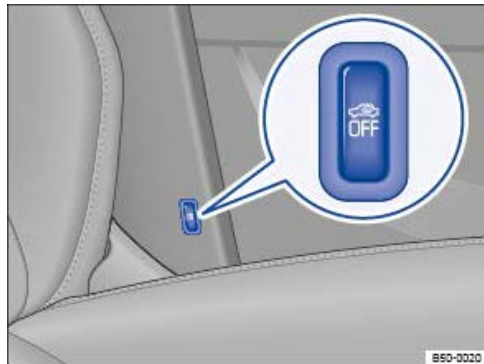
Fig. 72 Next to the driver seat: button for switching off the interior monitoring system and anti-tow alarm.
