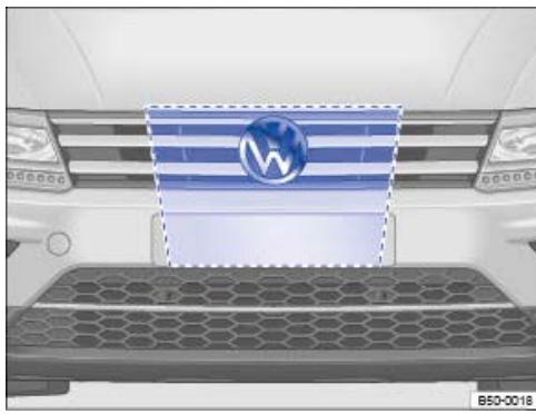
Fig. 158 In the radiator grille behind the Volkswagen badge: radar sensor and area around the radar sensor to be kept clear.
