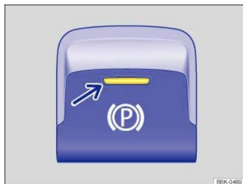
Fig. 173 In lower part of centre console: button for the electronic parking brake.
