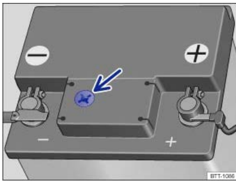
Fig. 263 A typical window on the top of the vehicle battery.
