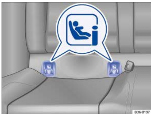
Fig. 26 On vehicle seat: markings identifying the ISOFIX anchoring points for child seats.
