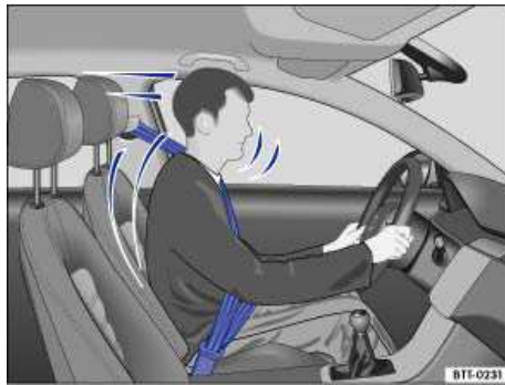
Fig. 77 Belted driver secured by the correctly worn safety belt in the event of a sudden braking maneuver.
