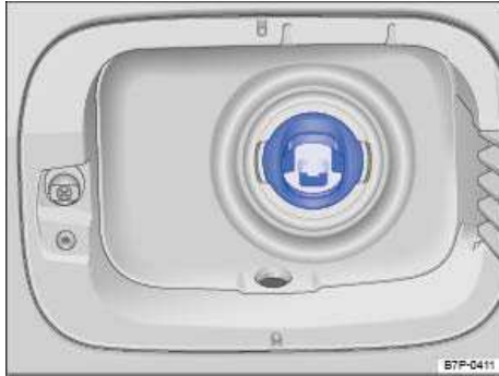
Fig. 178 With open fuel cap: Misfueling guard in the fuel filler neck.
