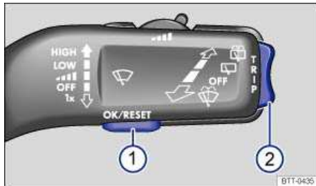
Fig. 16 Basic version (vehicles without menu control multi-function steering wheel): Control buttons 1 and 2 on the windshield wiper lever.
