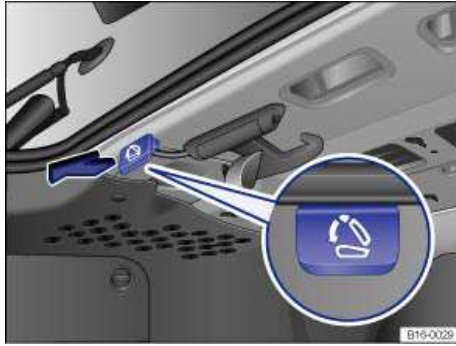
Fig. 115 On the left side of the luggage compartment: Release lever for the left-side rear seat backrest. The release lever for the right-side rear seat backrest is on the right side of the luggage compartment.
