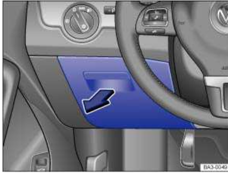
Fig. 135 On driver side: Storage compartment.
