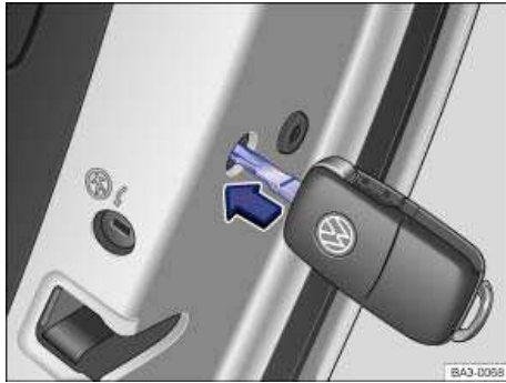
Fig. 198 On the front side of the right rear door: Manual vehicle locking with the key bit in the vehicle key.
