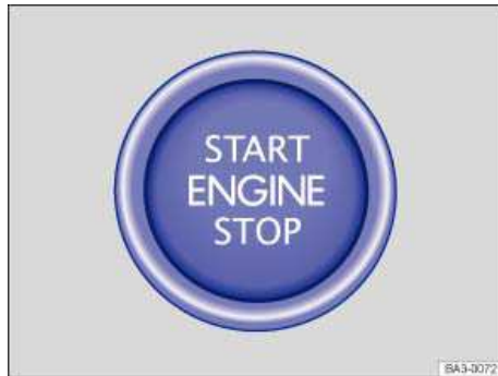
Fig. 151 In the center console: Starter button of the Keyless Access with push button start.
