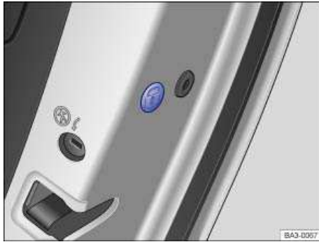
Fig. 197 On the front side of the right rear door: Emergency lock, covered by a rubber seal.
