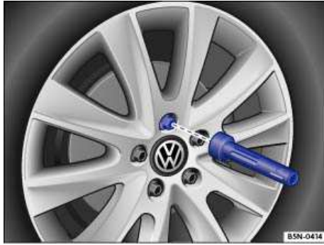
Fig. 213 Changing a wheel: remove previously loosened wheel bolts using the screwdriver handle.
