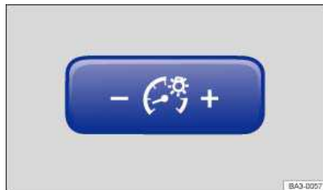
Fig. 103 To the left of the steering wheel: Control for instrument panel lighting.
