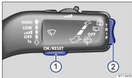
Fig. 18 Premium version (vehicles without menu control multi-function steering wheel): Control buttons 1 and 2 on the windshield wiper lever.
