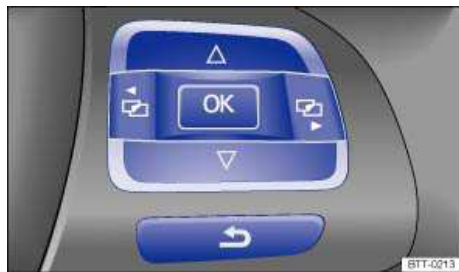
Fig. 17 Premium version (vehicles with menu control multi-function steering wheel): Buttons on the right side of the steering wheel.
