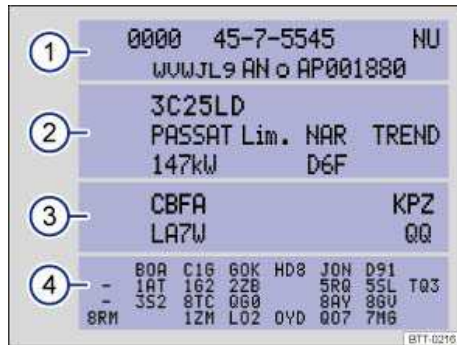
Fig. 20 Vehicle identification label: Shown in the example with engine identification code CBFA 3.
