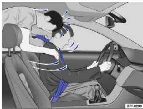
Fig. 76 Unbelted passengers in the rear seats are thrown forward on top of the belted driver.
