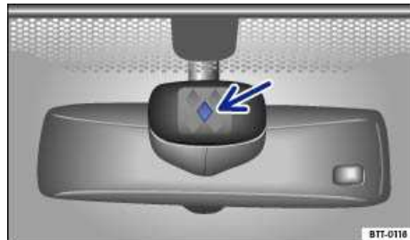
Fig. 109 Inside the front windshield above the inside mirror: Sensitive rain sensor surface.
