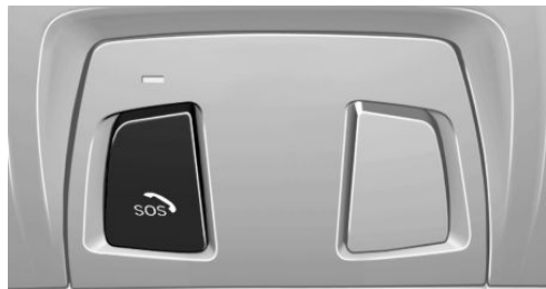
SOS button in the roofliner.
