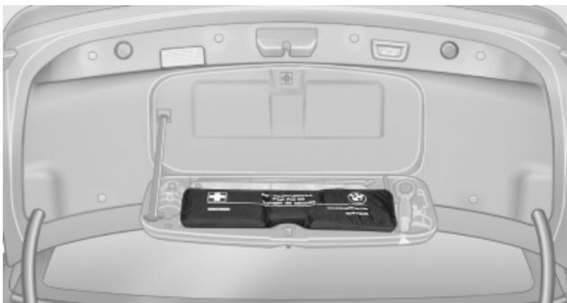
The first aid kit is located in the container on the inside of the trunk lid.
