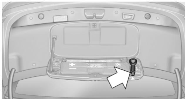
The screw-in tow fitting should always be carried in the vehicle. It can be screwed in at the front or rear of the BMW. It is located in the container on the inside of the trunk lid.
