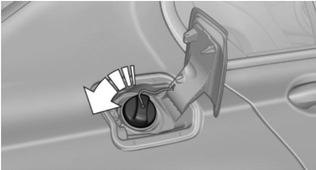
3. Place the fuel filler cap in the bracket attached to the fuel filler flap.
