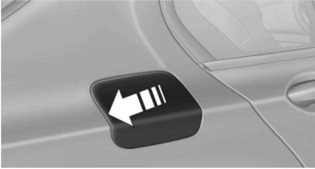
2. Turn the fuel filler cap counterclockwise.
