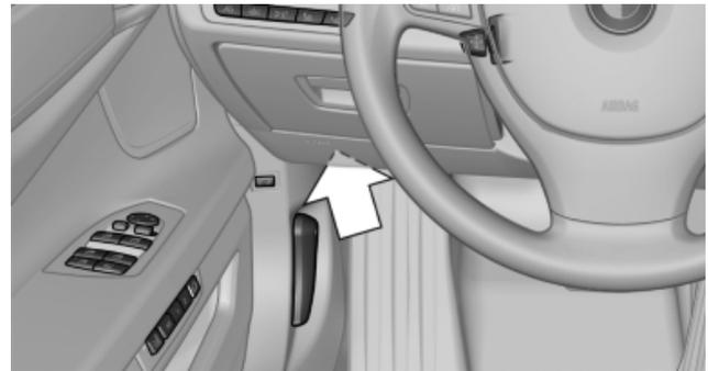
On the driver's side is an OBD socket for checking the primary components in the vehicle emissions.
