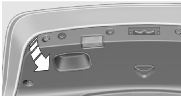
3. Replace the defective bulb.
