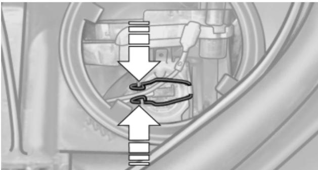
4. Release the holder and fold it upward.
