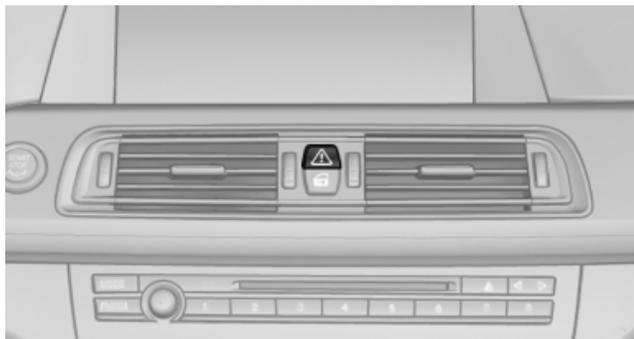
The button for the hazard warning flashers is located in the center console.
