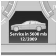
The system obtains information about the road safety and operational reliability of the vehicle and takes into account aspects such as a timely vehicle check. The aim is to optimize maintenance procedures with a view to reducing the cost of running the vehicle.
