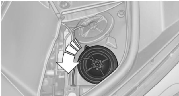
3. Squeeze the holder together and guide it downward.
