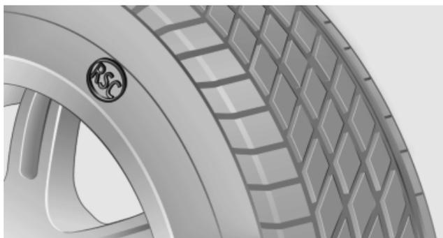
RSC label on the tire sidewall.
