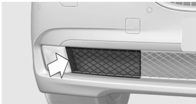
2. Remove the screw using a screw driver.
