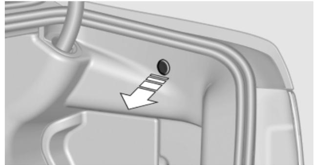
Pull the green knob with the fuel pump symbol. This releases the fuel filler flap.
