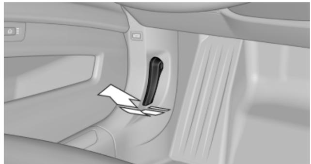
2. Press the release handle and open the hood.
