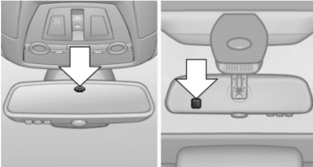
Photocells are used for control:
