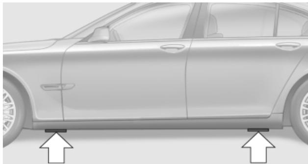
The jacking points for the vehicle jack are located in the positions shown.
