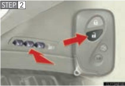
While the desired button (“1”, “2” or “3”) press
