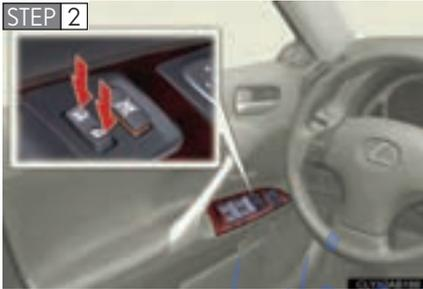
**STEP 2** Shift the shift lever to P or N, press and hold the driver's door lock switch (
