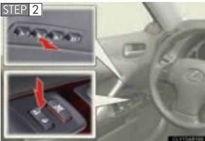
While pressing the desired button (“1”, “2” or “3”), press the lock or unlock side on the driver's door lock switch until the signal beeps.
