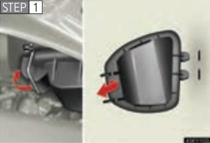
Release the lock and remove the cover.
