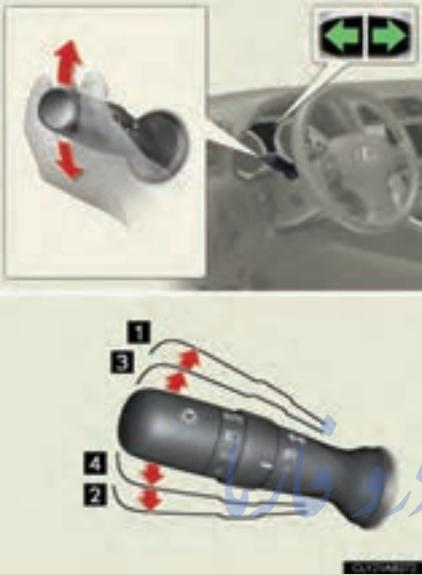
The diagram illustrates the operation of a turn signal lever. The top left shows a close-up of the lever with red arrows indicating its movement: up for right turn and down for left turn. The top right shows the lever in a car's interior with green arrows on the dashboard indicating the direction of the flashing lights. The bottom part shows a detailed view of the lever with numbered callouts: 1 (right turn), 2 (left turn), 3 (lane change), and 4 (lane change).
