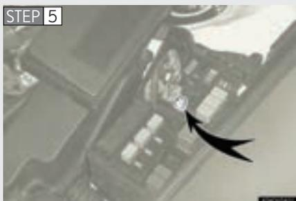
Remove the fuse with the pull-out tool.
