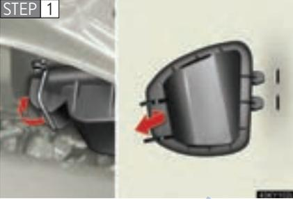
Release the lock and remove the cover.
