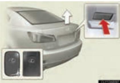
Press the button to unlock the trunk.
