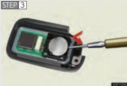
Remove the depleted battery.
