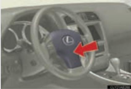
To sound the horn, press on or close to the
