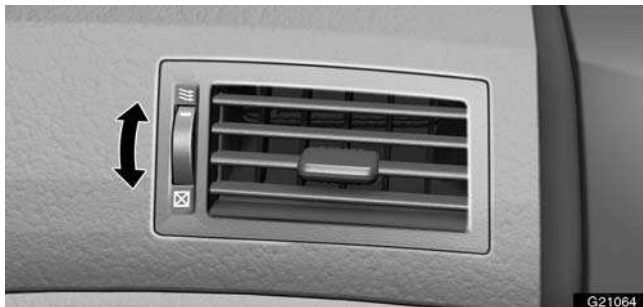
► Side vents (front passenger's side)
