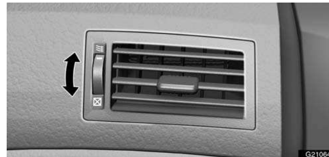
► Side vents (front passenger's side)
