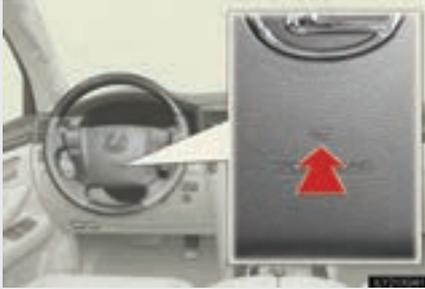
To sound the horn, press on or close to the
