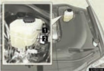
The brake fluid level should be between the “MAX” and “MIN” lines on the tank.
