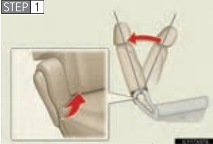
Fold the seatback while pulling the seatback angle lever. Return the seatback and secure it at the first lock position. (→P. 66)
