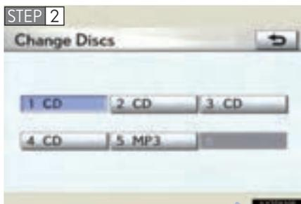
Touch the desired disc on the screen or press  $\wedge$  or  $\vee$  on
