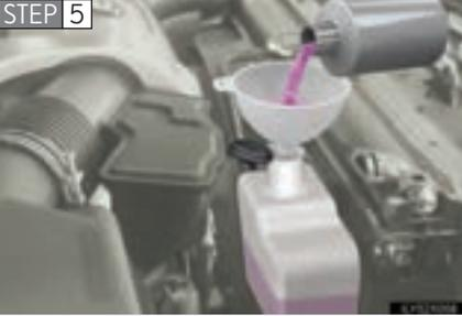
Add engine coolant if necessary.
