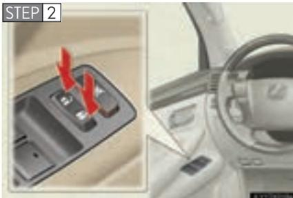
Shift the shift lever to "P" or "N", and press and hold the driver's door lock switch (
