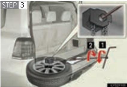
Insert the jack handle extension into the lowering screw.
