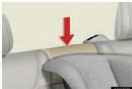
Lower the head restraint to the lowest position.
