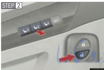
While pressing the desired button (“1”, “2” or “3”), press
