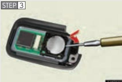
Remove the depleted battery.
