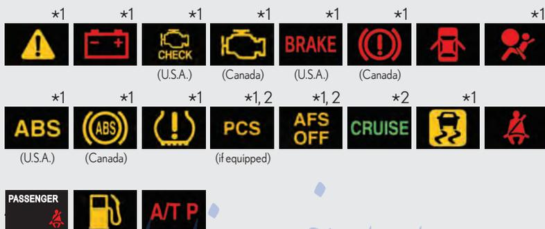
\*1: These lights turn on when the “ENGINE START STOP” switch is turned to IGNITION ON mode to indicate that a system check is being performed. They will turn off after the engine is started, or after a few seconds. There may be a malfunction in a system if a light does not come on, or if the lights do not turn off. Have the vehicle inspected by your Lexus dealer for details.
