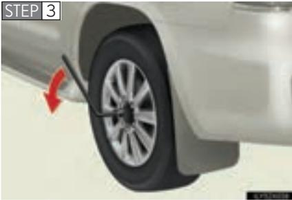
Slightly loosen the wheel nuts (one turn).
