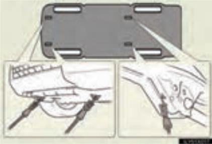
If your Lexus is transported by a flat bed truck, it should be tied down at the locations shown in the illustration. When attaching the hooks to the rear of the vehicle, make sure to attach them to the inside of the vehicle.
