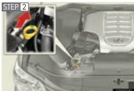
Hold a rag under the end and pull the dipstick out.
