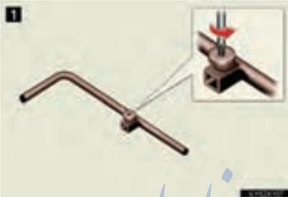
1 Loosen the screw using a screwdriver.
