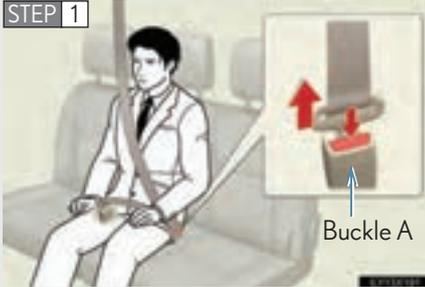
Push the release button on buckle A
