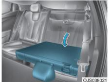
4. Remove the belt from the clip (1) and pull up the seatback folding lever (2), then fold the seat toward the front of the vehicle.
