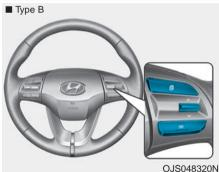
To change the trip mode, toggle the "\( \), \( \)" switch on the steering wheel.
