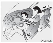
Your vehicle is equipped with driver's and front passenger's Pre-tensioner Seat Belts (Retractor Pretensioner and Emergency Fastening Device System). The purpose of the pre-tensioner is to make sure the seat belts fit tightly against the occupant's body in certain frontal or side collision(s). The Emergency Fastening Device System may be activated in certain crashes where the frontal collision(s) is severe enough, together with the air bags.
