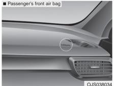
The purpose of the SRS is to provide the vehicle's driver and front passengers with additional protection than that offered by the seat belt system alone. The advanced SRS offers the ability to control the air bag inflation within two levels. A first stage level is provided for moderate-severity impacts. A second stage level is provided for more severe impacts.
