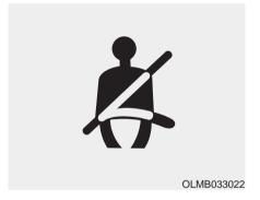
As a reminder to the driver, the seat belt warning light will illuminate for approximately 6 seconds each time you place the ignition switch to the ON position regardless of belt fastening. At this time, if the seat belt is not fastened a warning chime will sound for 6 seconds.
