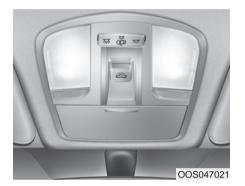
The sunroof can only be opened, closed, or tilted when the ignition switch is in the ON position.
