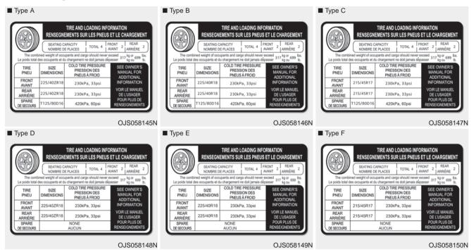
The label located on the driver's door sill gives the original tire size, cold tire pressures recommended for your vehicle, the number of people that can be in your vehicle and vehicle capacity weight.
