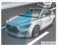
The Lane Keeping Assist (LKA) system helps detect lane markers on the road with a camera at the front windshield, and assists the driver's steering to help keep the vehicle between lanes.
