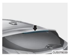
If the high mounted stop lamp does not operate, have the vehicle checked by an authorized HYUNDAI dealer.
