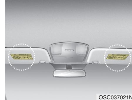
Air bag warning labels, some required by the Canada Motor Vehicle Safety Standards (CMVSS), are attached to the sun visor to alert the driver and passengers of potential risks of the air bag system.
