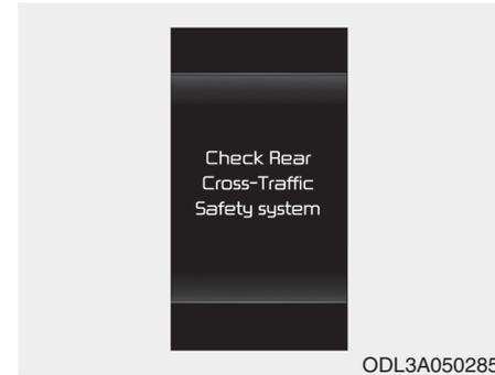
When Rear Cross-Traffic Safety is not working properly, the 'Check Rear Cross-Traffic Safety system' warning message will appear on the cluster, and the function will turn off automatically, or the function will be limited. In this case, have your vehicle inspected by an authorized Kia dealer.
