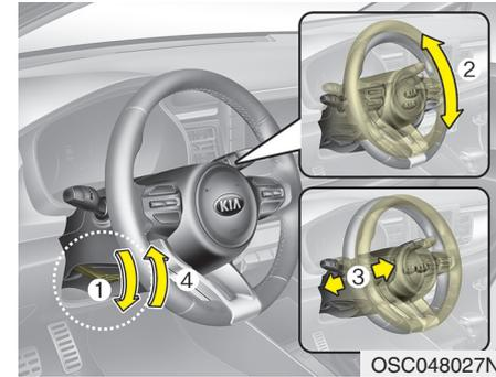
To change the steering wheel angle, pull down the lock release lever (1), adjust the steering wheel to the desired angle (2), then pull up the lock-release lever to lock (3) the steering wheel in place. Be sure to adjust the steering wheel to the desired position before driving.
