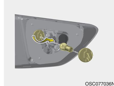
3. Remove the socket from the assembly by turning the socket counterclockwise until the tabs on the socket align with the slots on the assembly.
