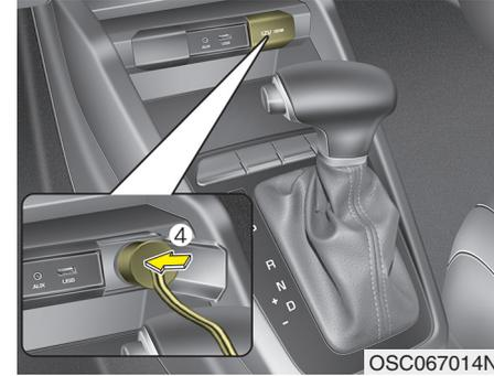
9. Connect between compressor and the vehicle power outlet (4) using the cable and connectors.
