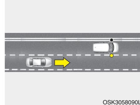
Blind-Spot Collision Warning help detects and informs the driver that a vehicle is approaching at high speed from the blind spot area.
