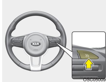
1. Press the Driving Assist (
