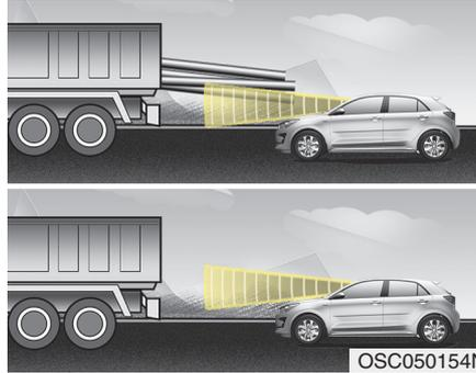
When the vehicle in front has heavy loading extended rearward, or when the vehicle in front has higher ground clearance, it may induce a hazardous situation. Always pay attention to road and driving conditions, while driving and, if necessary, depress the brake pedal to reduce your driving speed in order to maintain distance.
