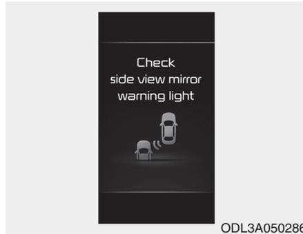
When the outside rearview mirror warning light is not working properly, the 'Check side view mirror warning light' warning message will appear on the cluster. In this case, have your vehicle inspected by an authorized Kia dealer.
