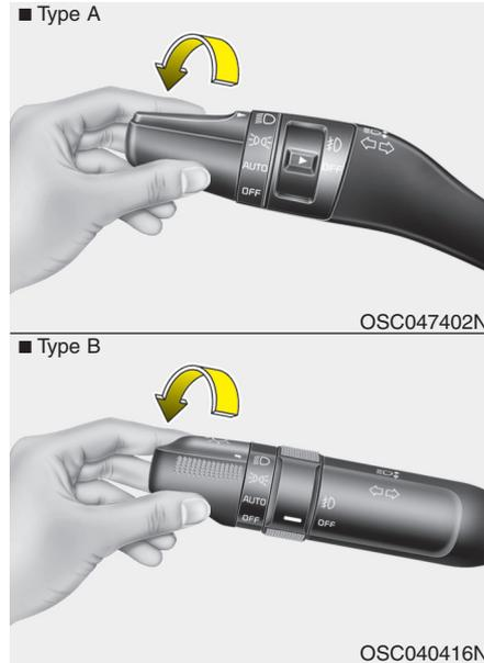
When the light switch is in the headlight position (4th position) the head, tail, position, license and instrument panel lights will turn ON.
