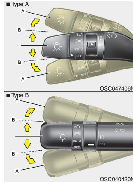
The ignition switch must be on for the turn signals to function. To turn on the turn signals, move the lever up or down (A). The green arrow indicators on the instrument panel indicate which turn signal is operating.
