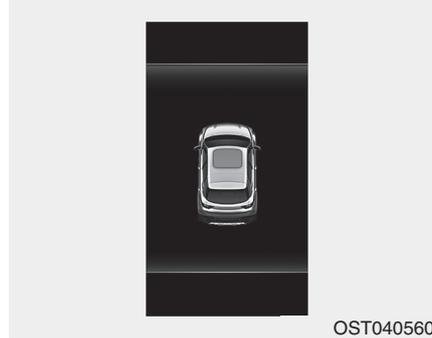
If the driver removes the ignition key (smart key: turns off the engine) and opens the driver-side door when the sunroof is not fully closed, the warning chime will sound for a few seconds and a warning image will appear on the LCD display.
