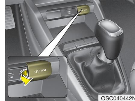
The power outlet is designed to provide power for mobile telephones or other devices designed to operate with vehicle electrical systems. The devices should draw less than 12V, 15A with the engine running.
