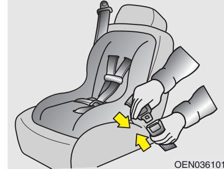
To install a child restraint system on the outboard or center rear seats, do the following:
