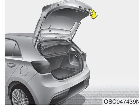
To close the liftgate, lower and push down the liftgate firmly. Make sure that the liftgate is securely latched.
