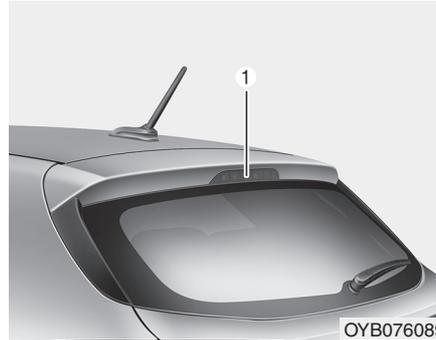
If the high mounted stop lamp (1) does not operate, have the vehicle checked by an authorized Kia dealer. A skilled technician should check or repair the high mounted stop lamp, for it may damage related parts of the vehicle.
