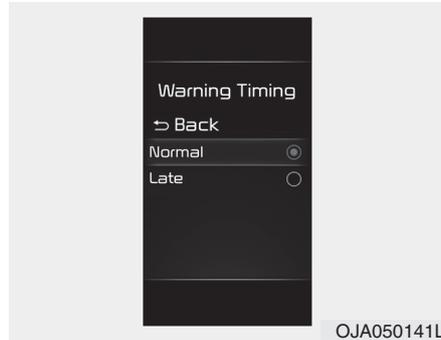
The driver can select the initial warning activation time in the User Settings in the LCD display by selecting "User Settings → Driver Assistance → Warning Timing". When the vehicle is first delivered, warning timing is set to 'Normal'. If you change the warning timing, the warning time of other Driver Assistance functions may change. Make sure to check the warning timing before changing it.
