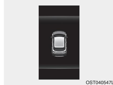
The warning message will appear on the LCD display when hood is open. The warning chime will operate when the vehicle is being driven at or above 3 km/h (2 mph) with the hood open.
