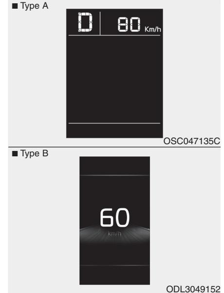
This mode displays the current speed of the vehicle.
