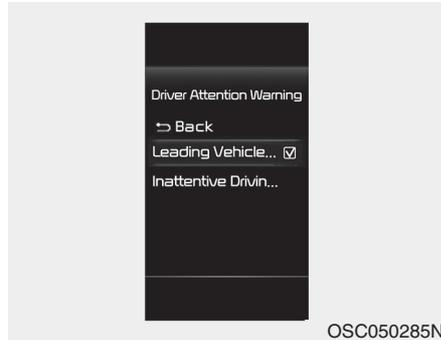
If 'Leading Vehicle Departure Alert's is selected, the function will inform the driver when the front vehicle departs from a stop.
