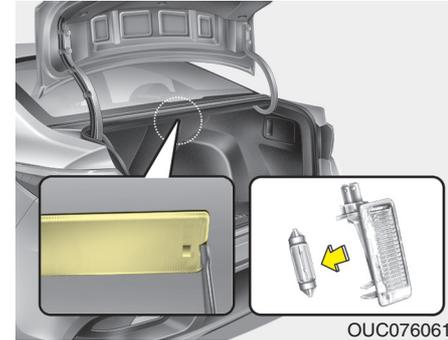
1. Using a flat-blade screwdriver, gently pry the lens cover from lamp housing.
