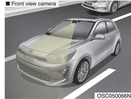
The front view camera is used as a detecting sensor to detect driving patterns and front vehicle departure while vehicle is being driven.
