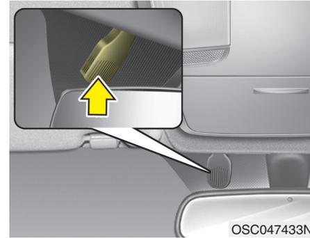
Auto defogging reduces the possibility of fogging up the inside of the windshield by automatically sensing the moisture inside the windshield and air flow toward the windshield can increase.
