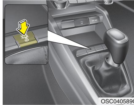
With the ignition switch or ENGINE START/STOP button in the ON position, pressing the heated steering wheel button warms the steering wheel. The indicator on the button will illuminate.
