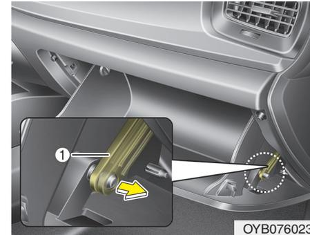
2. With the glove box open, pull the support strap (1).
