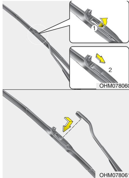
2. Lift up the wiper blade clip. Then pull down the blade assembly and remove it.
