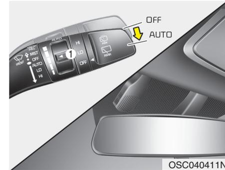
The rain sensor located on the upper end of the windshield glass senses the amount of rainfall and controls the wiping cycle for the proper interval. The more it rains, the faster the wiper operates. When the rain stops, the wiper stops.
