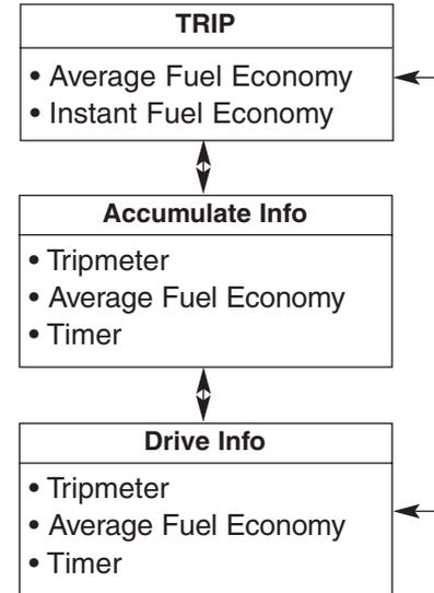
To change the trip mode, scroll the MOVE scroll switch (^/∨) in the trip computer mode.
