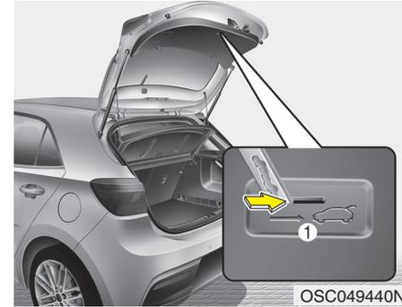
Your vehicle is equipped with the emergency liftgate safety release lever located on the bottom of the liftgate. If someone is inadvertently locked in the luggage compartment. The liftgate can be opened by doing as follows:
