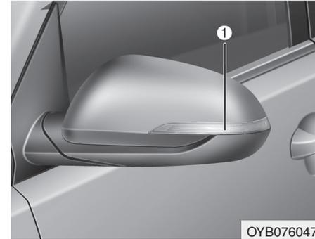
If the side repeater lamp (LED) (1) does not operate, have the vehicle checked by an authorized Kia dealer.
