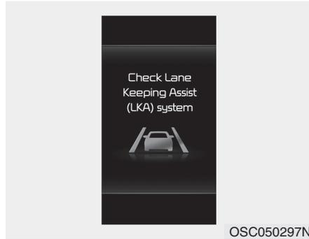
When Lane Keeping Assist is not working properly, the 'Check Lane Keeping Assist (LKA) system', warning message will appear and the yellow (LKA) indicator light will illuminate on the cluster. In this case, have your vehicle inspected by an authorized Kia dealer.
