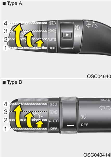
The light switch has a Headlight and a Parking light position.
