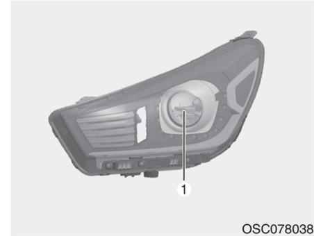
If the headlamp (Low/High beam) (1) does not operate, have the vehicle checked by an authorized Kia dealer.
