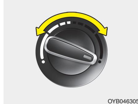
The temperature control knob allows you to control the temperature of the air flowing from the ventilation system. To change the air temperature in the passenger compartment, turn the knob to the right for warmer and hot air, or to the left for cooler air.
