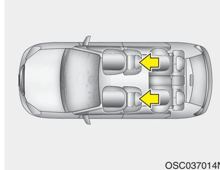
The driver's and front passenger's seats are equipped with a headrest for the occupant's safety and comfort. The headrest not only provides comfort for the driver and front passenger, but also helps protect the head and neck in the event of a collision.
