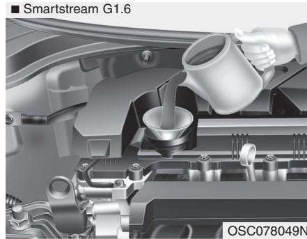
Check if the oil level is between the F-L line and refill it if the oil level is near the L line.
