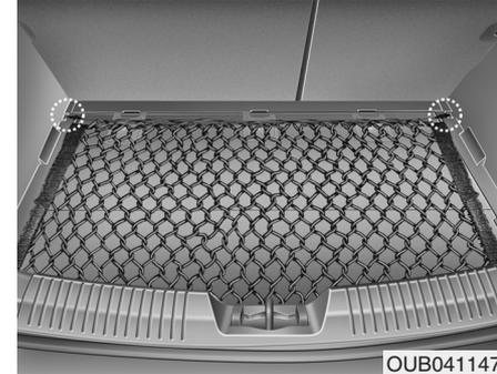
To keep items from shifting in the cargo area, you can use the 4 holders located in the cargo area to attach the luggage net (if equipped). If necessary, we recommend that you contact an authorized Kia dealer.
