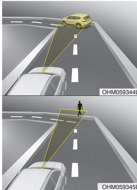
Forward Collision-Avoidance Assist may recognize a vehicle or pedestrian in the next lane or outside the lane when driving on a curved road.
