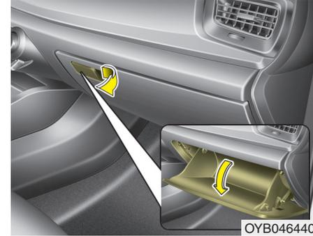
To open the glove box, pull the handle, and the glove box will automatically open. Close the glove box after use.
