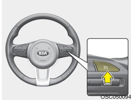
Press the Driving Assist
