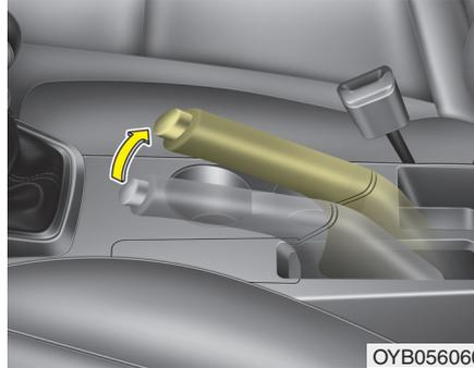
To engage the parking brake, first apply the foot brake and then without pressing the release button in, pull the parking brake lever up as far as possible. In addition it is recommended that when parking the vehicle on a gradient, the shift lever should be positioned in the appropriate low gear for Manual Transmission vehicles or in the P (Park) position for Intelligent Variable Transmission vehicles.
