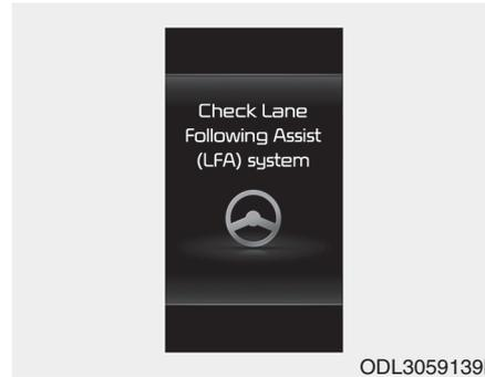
When Lane Following Assist is not working properly, the 'Check Lane Following Assist (LFA) system' warning message will appear on the cluster.
