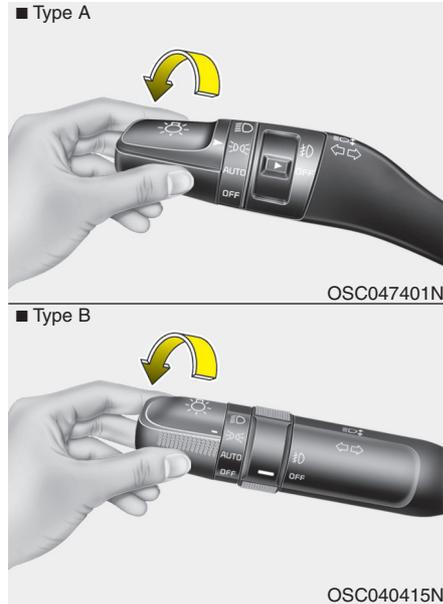
When the light switch is in the parking light position (3rd position), the tail, position, license and instrument panel lights will turn ON.
