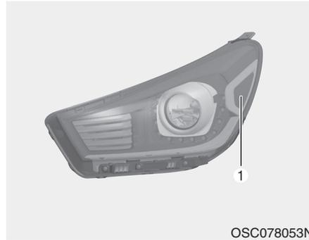
If the Side marker (LED) (1) does not operate, have the vehicle checked by an authorized Kia dealer.
