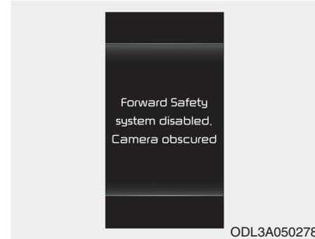
In this case, a warning message will appear to notify the driver. Remove the foreign substances to allow FCA to function normally.
