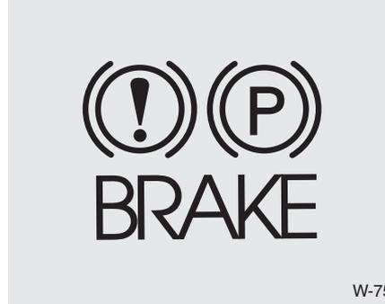
Check the brake warning light by turning the ignition switch or ENGINE START/STOP button ON (do not start the engine). This light will illuminate when the parking brake is applied with the ignition switch or ENGINE START/STOP button in the START or ON position.
