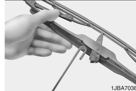
2. Compress the clip (1) and slide the blade assembly downward (2).
