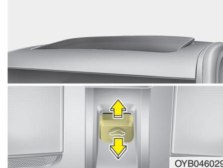
To tilt open the sunroof, push the sunroof control lever upward until the sunroof moves to the desired position.
