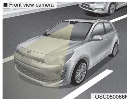
The front view camera is used as a detecting sensor to detect lane markings.
