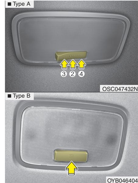
To turn the room lamp ON or OFF, push the switch.
