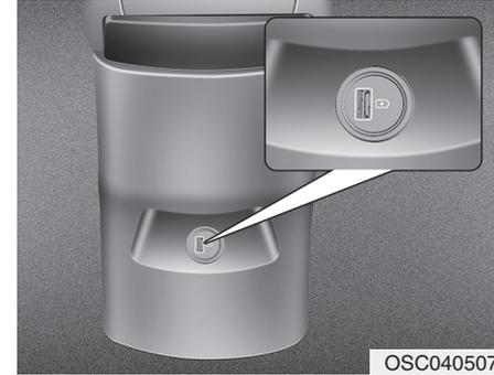
The USB charger is designed to recharge batteries of small size electrical devices using a USB cable. The electrical devices can be recharged when the ignition switch is in ACC/ON/START position.
