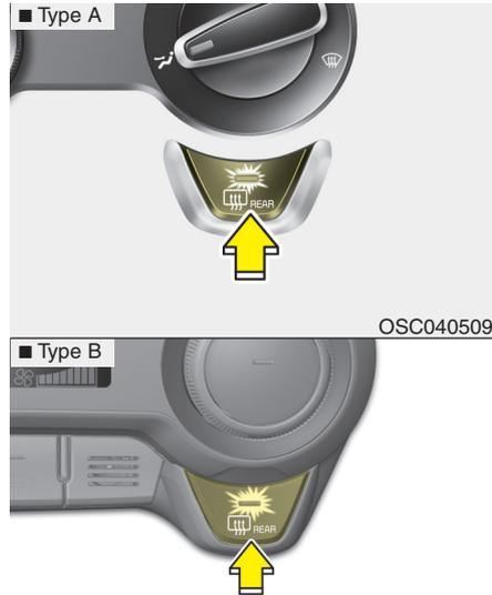
The defroster heats the window to remove frost, fog and thin ice from the interior and exterior of the rear window, while the engine is running.
