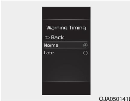
The driver can select the initial warning activation time in the User Settings in the instrument cluster LCD display.
