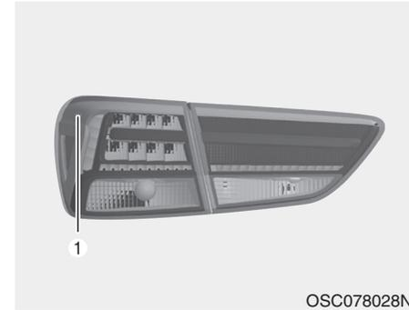
If the Side marker (LED) (1) does not operate, have the vehicle checked by an authorized Kia dealer.
