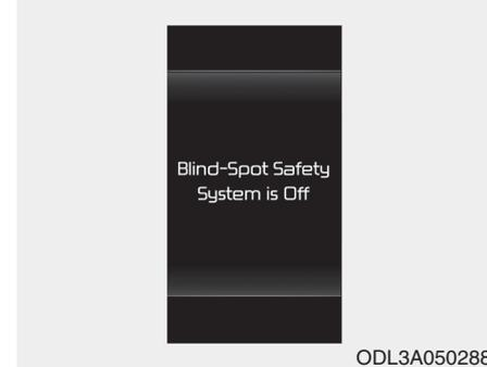
When the engine is restarted with the function off, the 'Blind-Spot Safety System is Off' message will appear on the cluster.
