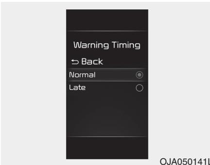
With the ignition switch or ENGINE START/STOP button in the ON position, select 'Driver Assistance → Warning Timing' from the User Settings to change the initial warning activation time for Blind-Spot Safety system.
