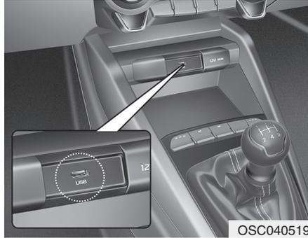
You can use an USB port to plug in an USB.
