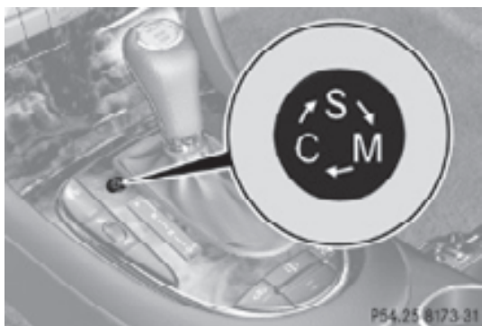
Program mode selector switch on CLS 63 AMG
