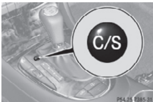
Program mode selector switch
