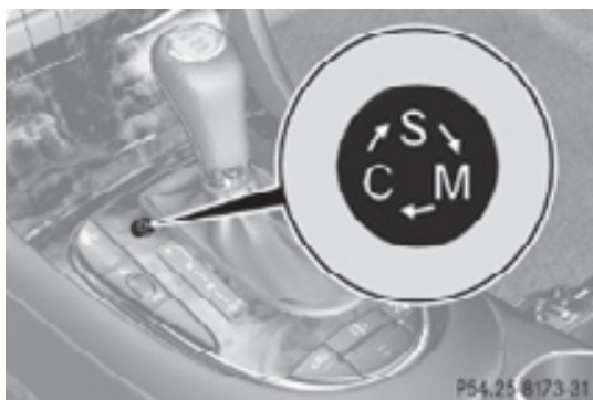
Program mode selector switch on CLS 63 AMG
