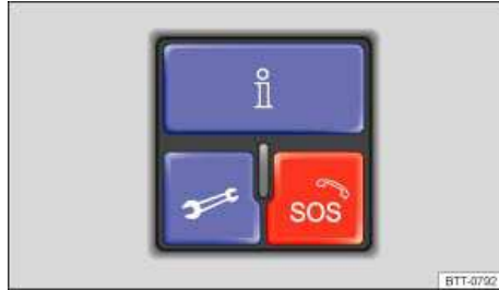
Fig. 18 In the roof console: 3-button module to access Volkswagen Car-Net service operators
