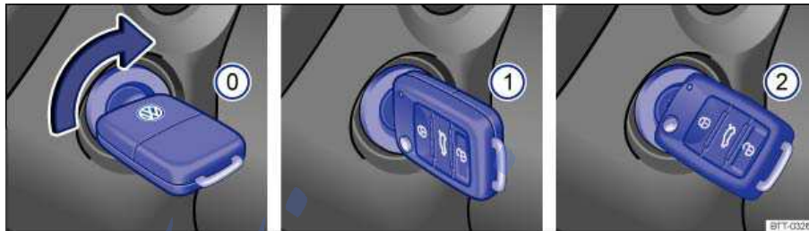
Fig. 111 In the ignition switch: Vehicle key positions.
