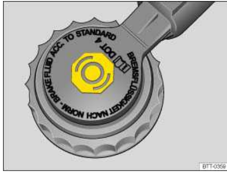
Fig. 123 In the engine compartment: Brake fluid reservoir cap.
