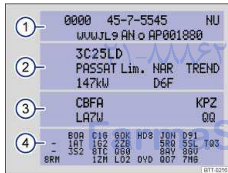
Fig. 19 Vehicle identification label: Shown in the example with engine identification code CBFA 3.
