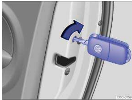
Fig. 154 On the edge of the passenger door: Manually locking the door with the vehicle key.
