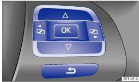
Fig. 17 Right side of the multi-function steering wheel (if equipped): Controls for the menus in the instrument cluster.
