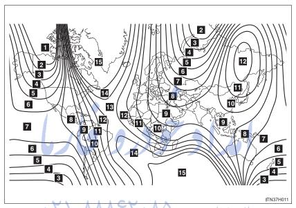
The direction display deviates from the true direction determined by the earth's magnetic field. The amount of deviation varies depending on the geographic position of the vehicle.
