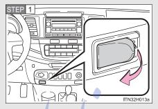
Open the cover and connect the portable audio device
