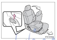
Pull the seatback angle adjustment lever and fold down the seatback. The seat will slide forward.
