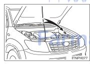
The manufacturer's label is located beside the engine compartment.
