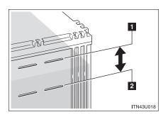
Check that the level is between the upper and lower lines.
