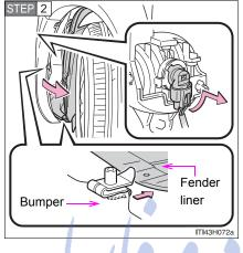
Partly remove the fender liner and turn the bulb base counter-clockwise.
