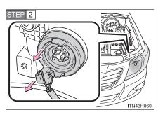
Unplug the connector and remove the rubber cover.
