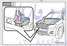
Pull up the auxiliary catch lever and lift the hood.
