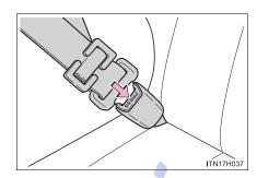
2-point type seat belt (if equipped): Push the buckle release button.
