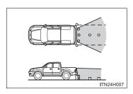
The area covered by the camera is limited. Objects which that are close to either corner of the bumper or under the bumper cannot be seen on the screen.
