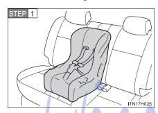
Place the child restraint system on the rear seat facing the front of the vehicle.
