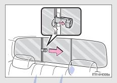
To open the back window, push the lock release lever and slide the back window.
