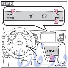
Press and hold the "INFO." or "DISP" button until a number (1 to 15) appears on the clock. Then press the "H" or "M" button, and referring to the map above, select the number of the zone where you are.
