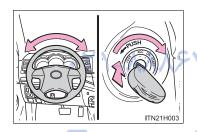
When starting the engine, the engine switch may seem stuck in the "LOCK" position. To free it, turn the key while turning the steering wheel slightly left and right.
