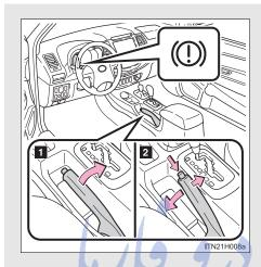
■ To set the parking brake, fully pull the parking brake lever while depressing the brake pedal.
