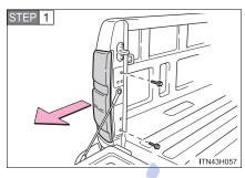
Remove the securing bolts and remove the unit.
