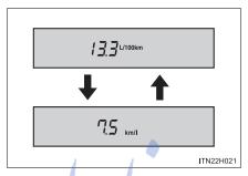
Unit for only the fuel consumption rate can be interchanged.
