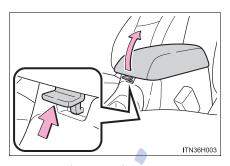
Lift the lid while pulling up the knob to release the lock.
