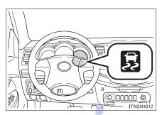
If the vehicle is in danger of slipping or if any of the drive wheels spins, the slip indicator flashes to indicate that the VSC/TRC systems are operating.
