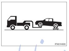
Vehicles with automatic transmission: Use a towing dolly under the rear wheels.
