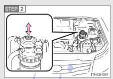
To bleed the fuel system, operate the priming pump until you feel more resistance.
