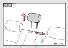
Remove the center head restraint.
