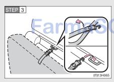
Anchor the strap to the bracket behind the rear seat.
