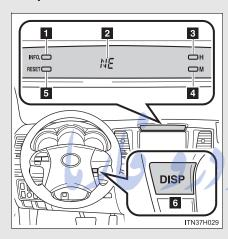
To turn the compass on, press the "INFO." or "DISP" button until the compass appears.  $(\rightarrow P. 185)$
