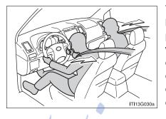
The pretensioner helps the seat belt to quickly restrain the occupant by retracting the seat belt when the vehicle is subjected to certain types of severe frontal collision or side collision (vehicles with SRS side airbags and curtain shield airbags).
