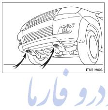
If a tow truck is not available in an emergency, your vehicle may be temporarily towed using a cable or chain secured to the emergency towing eyelet(s). This should only be attempted on hard surfaced roads for short distances at low speeds.
