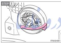
Release the bulb retaining spring.
