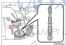
If the washer fluid level is at "LOW", add washer fluid.
