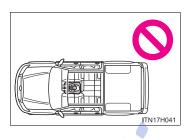
Vehicles with front bench seat: Do not install a child restraint system in the center position. This seat position is not designed to hold a child restraint system.
