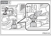
Add engine coolant if necessary.
