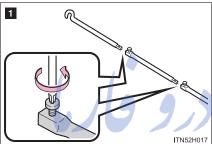
**1** Loosen the bolts using a screwdriver.
