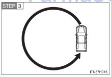
Drive the vehicle at 8 km/h (5 mph) or less in a circle until a direction is displayed.
