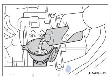
If any washer does not work, the washer tank may be empty. Add washer fluid.
