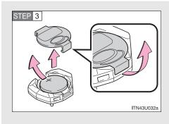
Remove the battery cover and the depleted battery.
