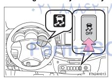
To turn the TRC system off, quickly press and release the button.
