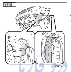
To allow enough working space, turn the steering wheel to the opposite side of the bulb to be replaced.
