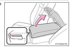
• When using the console box lid as an armrest, slide the console box lid forward as needed. Slide the lid forward while pulling up the lever.
