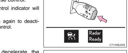
2 Accelerate or decelerate the vehicle to the desired speed, and push the lever down to set the speed.
