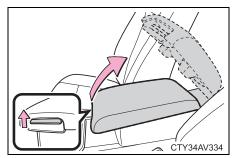
The console box is provided with a cutout that allows cables to be routed from the power outlet in the console box with the lid closed.
