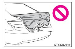
Do not attach any accessories other than genuine Toyota parts to the trunk lid. Such additional weight on the trunk lid may cause the lid to suddenly shut again after it is opened.
