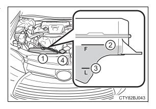
5 Add engine coolant if necessary.
