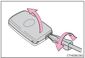
Remove the depleted battery.
