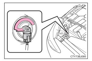
2 Pull the bulb out while pressing the lock release of the connector.
