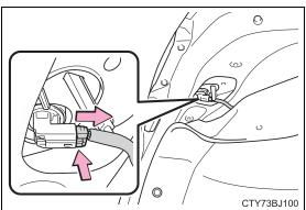
3 Turn the bulb base counter-clockwise.
