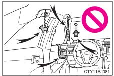
Do not hang coat hangers or other hard objects on the coat hooks. All of these items could become projectiles and may cause death or serious injury, should the SRS curtain shield airbags deploy.
