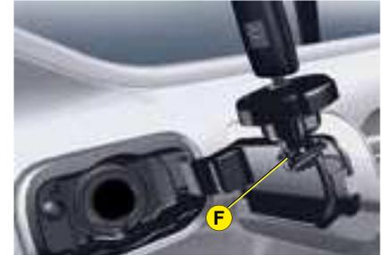
To open the fuel flap, press on the top left part of it, then pull from the edge.
