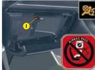
In order to be able to use a rear-facing child seat in the front passenger's seat position, it is imperative to deactivate the passenger's airbag.
