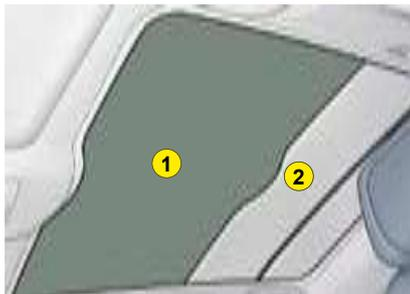
This device comprises a tinted glass panoramic surface **1** to improve brightness and vision in the passenger compartment.
