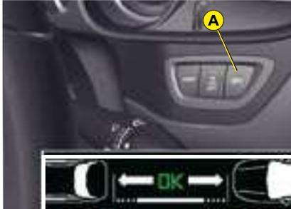
You can select the “Parking Space Sensor” by pressing button **A**, which flashes when next to the space to be measured, with a speed lower than 20 km/h (12 mph) and at a distance of less than 1.5 m from the space.
