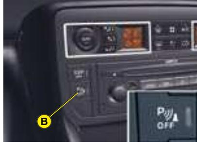
You can activate/deactivate the parking assistance by pressing button **B**. When the parking assistance is inactive, the warning lamp on button **B** is lit up.
