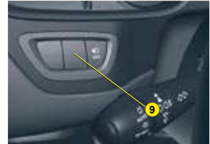
**9** Programmable heating system warning lamp.
