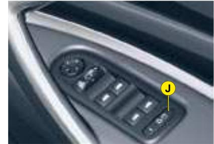
This deactivates the controls in the rear of the vehicle, both for the rear windows and for opening the rear doors from the inside. The electric child safety device is activated by pressing on button **J**.
