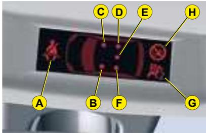
The seat belt fastened/unfastened status for each seat category is indicated by the lighting or flashing of the warning lamps linked to each position:
