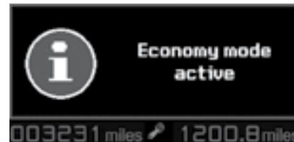
When the engine is stopped, some functions (audio system, screen wipe, electric windows, sunroof, electric seats, telephone, video, interior lighting etc.) are only electrically supplied for a maximum period of 30 minutes, to avoid discharging the battery.
