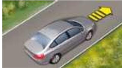
**On an ascending slope, with the vehicle stationary, the vehicle is held for a brief moment when you release the brake pedal:**
