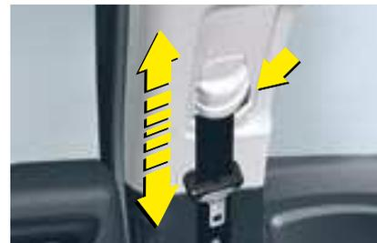
The **correct positioning** of the belt strap is **through the middle of the shoulder**. See "Seat belts".
