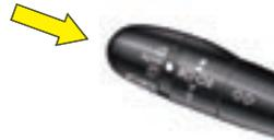
press on the voice recognition button. Activation of the function is confirmed by a beep and by the opening of a window on the display.
