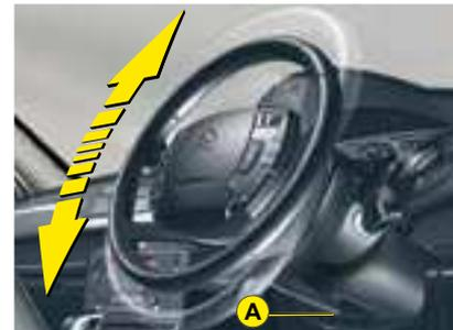
**With the vehicle at rest**, unlock the steering wheel by pushing control A forwards.
