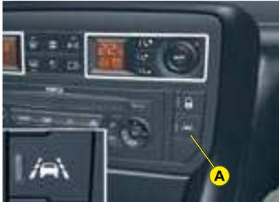
This driving assistance device warns you when you unwittingly cross a lane marking (either a continuous or a dotted line on the road surface). It is designed for use on motorways and dual carriageways, operating **only above speeds of approx. 80 km/h (50 mph)**.
