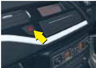
The hazard lamps can also be used with the ignition switched off.
