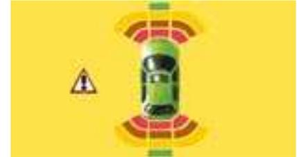
As the vehicle approaches the obstacle, the sound signal becomes more and more urgent and the shaded areas are displayed closer and closer to the vehicle.
