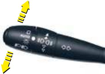
Move the stalk briefly upwards or downwards, without going beyond the resistance point; the direction indicators will flash 3 times.
