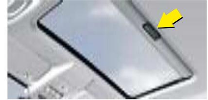
Your sun roof is fitted with a manually-operated blind.
