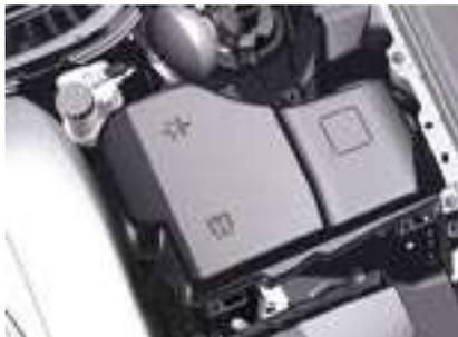
To access the fusebox under the bonnet, undo each screw by a 1/4 turn.
