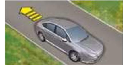
**On an descending slope, with the vehicle stationary and reverse gear engaged, the vehicle is held for a brief moment when you release the brake pedal.**
