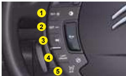
This driving assistance function allows you to drive at the speed of your choice **without the need to action the accelerator**. It is active over speeds of around 40 km/h (25 mph).
