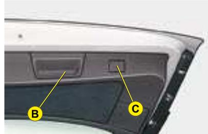
The tailgate automatically locks when the vehicle is moving at a speed of over 10 km/h (6 mph), even if automatic central locking is deactivated. It is unlocked when a door is opened or when the central locking button is pressed (at a speed of less than 10 km/h (6 mph)).
