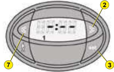
Press button **3** then buttons **2** or **7** in the next 10 seconds, until the desired start-up time is displayed.
