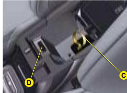
9. Make sure that you position the strap back in its location **C**. If not, the application of the parking brake will not be possible. Contact a CITROËN dealer.
