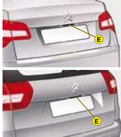
Press upwards on the lever **E**.
