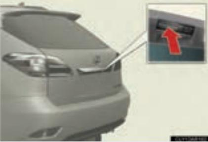
When the back door is unlocked: Press the back door opener button.
