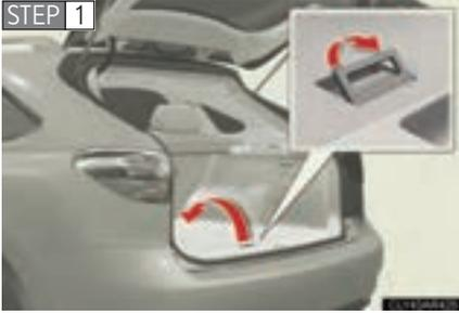
Pull the lever upward to fold back the front part of the deck board.
