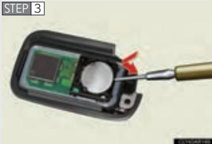
Remove the depleted battery.
