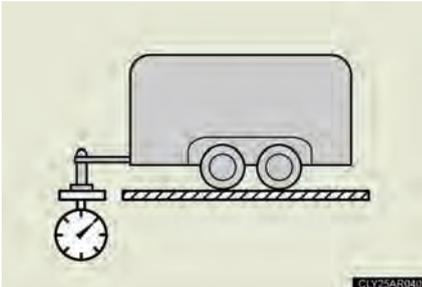
The load placed on the trailer hitch ball. (→P. 278)
