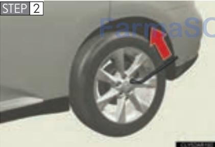
Slightly loosen the wheel nuts (one turn).
