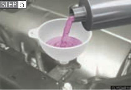
Add engine coolant if necessary.
