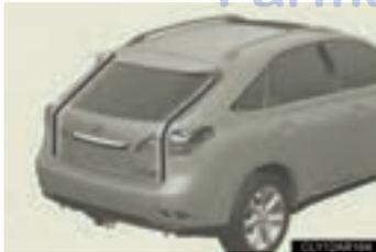
Sensors are attached to the left and right sides of the power back door. If these sensors detect an obstruction while the power back door is closing, the jam protection function will return the door to the fully open position.
