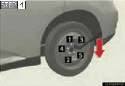
**STEP 4** Firmly tighten each wheel nut two or three times in the order shown in the illustration.
