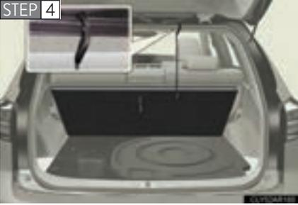
Use the hook to secure the deck board as shown in the illustration.
