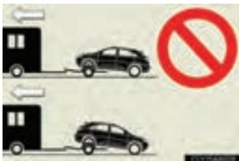
AWD models: Never tow this vehicle with any of the wheels on the ground. This may cause serious damage to the transmission and Active Torque Control 4WD system.
