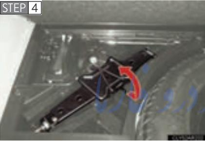
Remove the jack after removing the hook.
