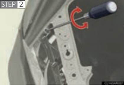
Turn bolt B the same number of turns and in the same direction as in step 1 using a Phillips-head screwdriver.
