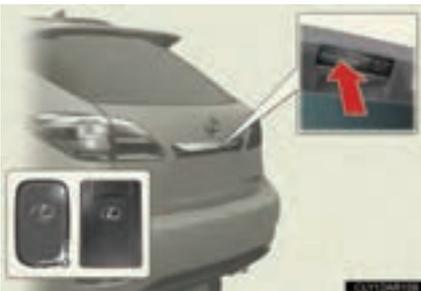
Press the button to unlock the door.
