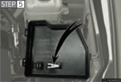
Remove the fuse with the pull-out tool.
