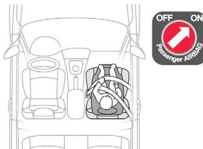
When a "forward facing" child seat is installed on the **front passenger seat**, adjust the vehicle's seat to the intermediate longitudinal position with the seat backrest straightened and leave the passenger's front airbag activated.
