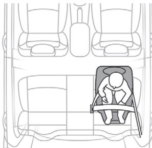
**!** When a "rearward facing" child seat is installed **on a rear passenger seat**, move the vehicle's front seat forward and straighten the backrest so that the "rearward facing" child seat does not touch the vehicle's front seat.
