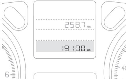
The total and trip distances are displayed for thirty seconds when the ignition is switched off, when the driver's door is opened and when the vehicle is locked or unlocked.
