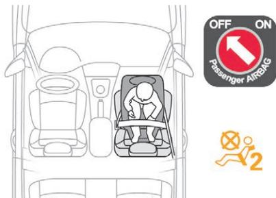
When a "rearward facing" child seat is installed on the **front passenger seat**, adjust the seat to the intermediate longitudinal position, with the backrest straightened.
