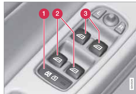
Driver's door control panel.
