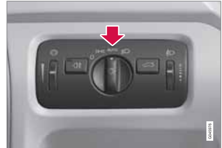
Light switch in position AUTO .
