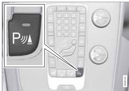
On/Off for the sensors for parking assistance and CTA 1 .
