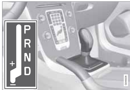
D: Automatic gear positions. +/-: Manual gear positions.
