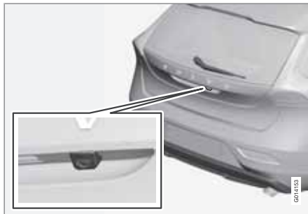
Camera location next to the opening handle.
