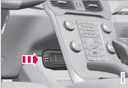
Handheld unit storage and charging station.
