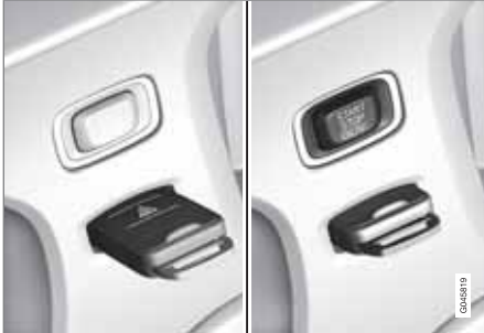
Ignition switch with remote control key extracted/inserted.
