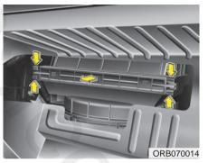
Remove the climate control air filter cover while pressing the lock of the cover.
