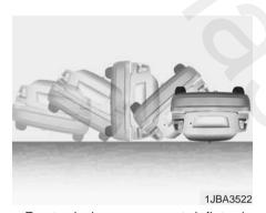
Front air bags may not inflate in rollover accidents because air bag deployment would not provide additional protection to the occupants.
