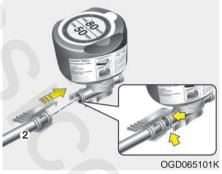
2. Connect the filling hose (2) onto the connector of the sealant bottle.
