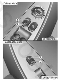
With central door lock switch (if equipped)
