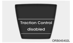
Press the ESC OFF button shortly (ESC OFF indicator light and message illuminates). At this state, the engine control function does not operate. In other words, the traction control function does not operate but only the brake control function operates.
