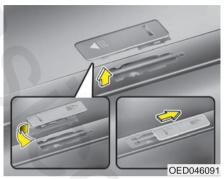
Rotate the cover half way and insert the cover on the roof hole as the illustration.
