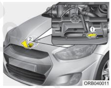
2. Go to the front of the vehicle, raise the hood slightly, push the secondary latch (1) to the left and lift the hood (2).
