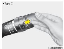
Push the lever away from you to spray rear washer fluid and to run the rear wipers 1~3 cycles. The spray and wiper operation will continue until you release the lever
