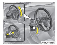
To change the steering wheel angle and height, pull down the lock release lever (1), adjust the steering wheel to the desired angle (2) and height (3), then pull up the lock-release lever to lock the steering wheel in place. Be sure to adjust the steering wheel to the desired position before driving.
