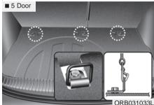
Securing a child restraint seat with "Tether Anchor" system
