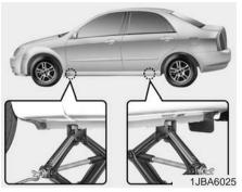
Place the jack at the front or rear jacking position closest to the tire you are changing. Place the jack at the designated locations under the frame
