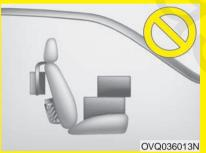
Never put a heavy load, an active electronic device or blanket in the front passenger seat or seatback pocket.
