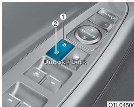
When pressing the (🔒) portion (1) of the switch, all vehicle doors will lock.
