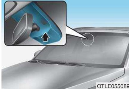
The SLIF displays the speed limit information and no-overtaking restriction through the instrument cluster and the navigation. The SLIF reads the traffic signs through the camera, which is attached on the upper part of the inner front windshield.
