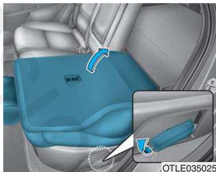
5. To use the rear seat, lift and push the seatback rearward by lifting up the front portion of the folding lever. Push the seatback firmly until it clicks into place. Make sure the seatback is locked in place.
