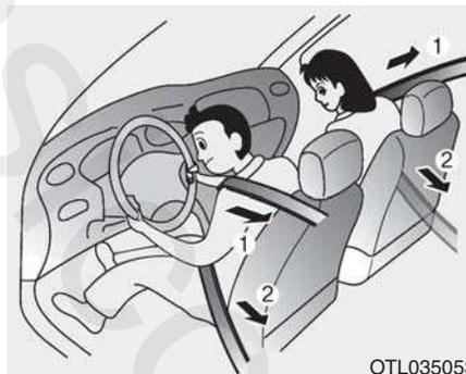
Your vehicle is equipped with driver's and front passenger's Pre-tensioner Seat Belts (Retractor Pretensioner and Emergency Fastening Device (EFD)). The purpose of the pre-tensioner is to make sure the seat belts fit tightly against the occupant's body in certain frontal collisions. The pre-tensioner seat belts may be activated in crashes where the frontal collision is severe enough, together with the air bags.
