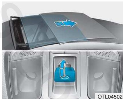
If you pull the sunroof control lever backward to the second detent, the sunshade will slide all the way open then the sunroof glass will slide all the way open. To stop the sunroof movement at any point, pull or push the sunroof control lever momentarily.
