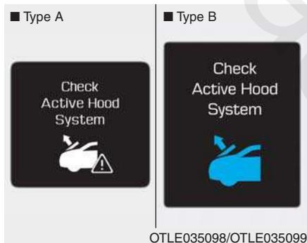
The warning message appears on the LCD display, when there is a malfunction with the active hood lift system.
