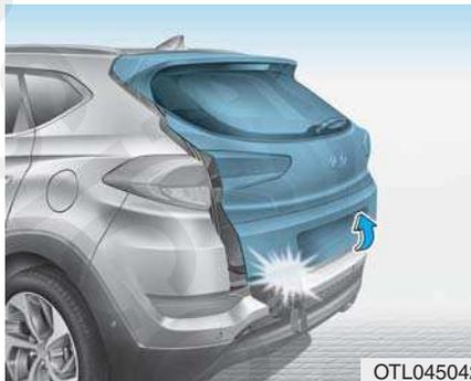
During power opening and closing if the power tailgate is blocked by an object or part of the body, the power tailgate will detect the resistance.
