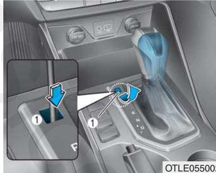
1. Place the ignition switch in the LOCK/OFF position.
