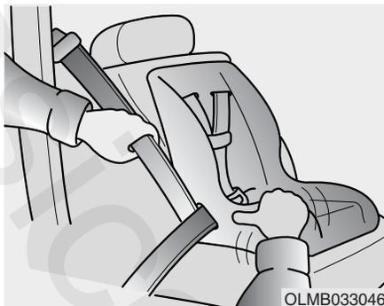
3. Remove as much slack from the belt as possible by pushing down on the Child Restraint System while feeding the shoulder belt back into the retractor.
