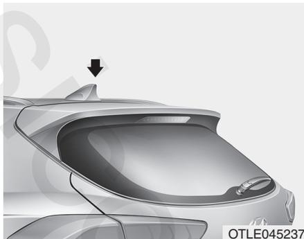
The shark fin antenna receives transmitted data. (for example: GPS and DAB signals)
