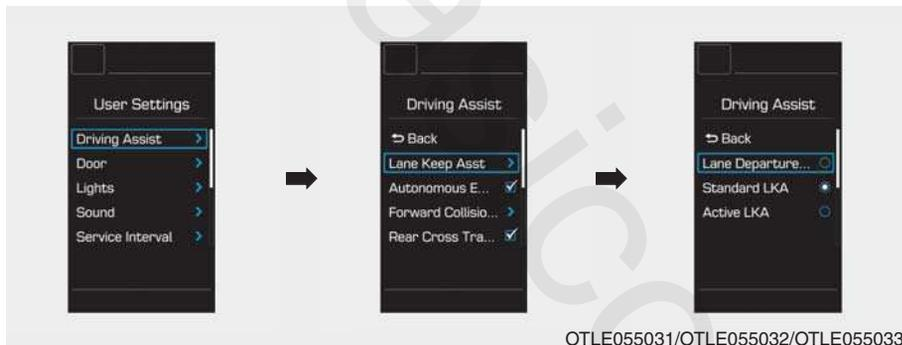
The driver can change LKAS to Lane Departure Warning System (LDWS) or change the LKAS mode between Standard LKA and Active LKA from the User Settings mode on the LCD display. The system is automatically set to Standard LKA if a function is not selected.
