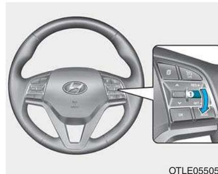
3. Push the lever (1) down (SET-), and release it. The SET indicator light will illuminate.
