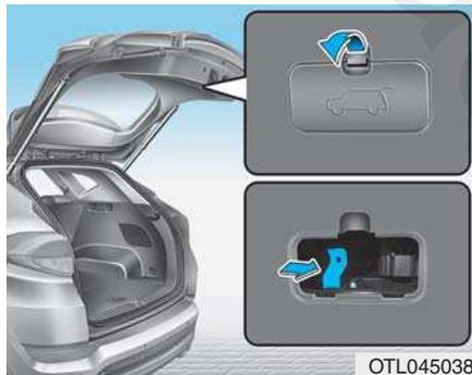
Your vehicle is equipped with the emergency tailgate safety release lever located on the bottom of the tailgate. When someone is inadvertently locked in the luggage compartment. The tailgate can be opened by doing as follows:
