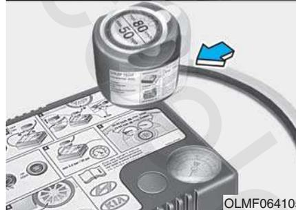
6. Ensure that the compressor is switched off, position 0.
